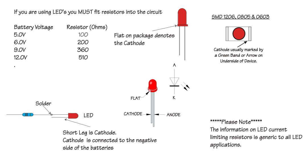
The Resistor can be placed in either Leg of the LED
